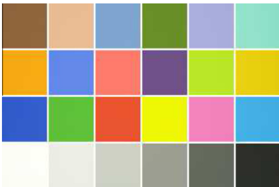
Fig. 2. The 24 reference colours of the X-Rite® color checker.
